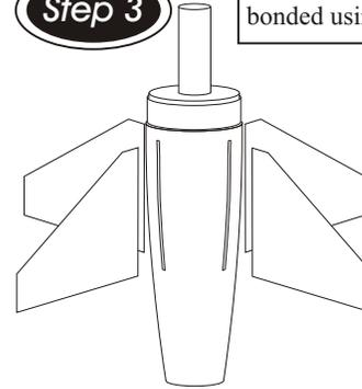
**1)** Apply a bead of epoxy to the root edge of a fin. Push the fin through the slot in the boat tail and against the motor mount tube. Make sure that the fin is
