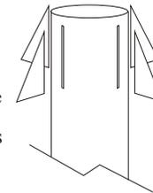
**2)** Apply an epoxy fillet to both sides of each fin. Carefully smooth the epoxy with your finger before it begins to gel. Allow the epoxy to set-up before rotating the rocket to do the next set of fins. Once the epoxy has fully cured, you should sand the fillet smooth with 180 grit sandpaper. Sanding will help the primer hold better to the epoxy.
