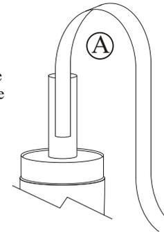
**B)** Epoxy the notched centering ring 1/2" down from the top of the motor mount tube. Apply a fillet to both sides of the ring.
