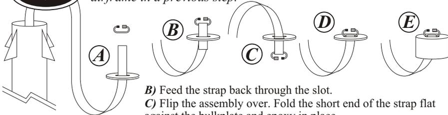
**A)** Pull the free end of the strap through the slot in the piston bulk plate. Slip the metal "D" ring over the strap.
