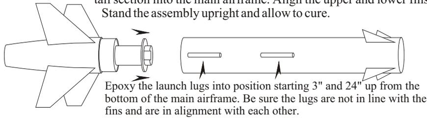
Epoxy the launch lugs into position starting 3" and 24" up from the bottom of the main airframe. Be sure the lugs are not in line with the fins and are in alignment with each other.
