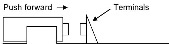
**Figure 3 - Battery End Clip Placement (Side View)**
