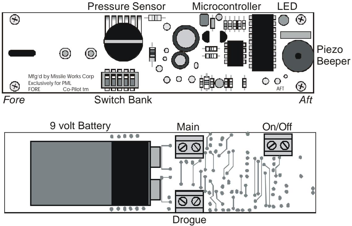
The switches are labeled 1 through 5. The ON/OFF position of the switches is also labeled, with an arrow on the switch pack itself pointing in the ON direction. The following table describes the switch functions and the corresponding modes of operation.
