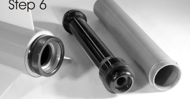
Push the motor all the way into the retainer. Apply a very small amount of grease onto the threads of the motor retainer to eliminate the potential for galling. Thread the retainer cap in place over the motor. Do not over-tighten the cap. Snugging it with your thumb and two fingers is enough. That's it, go fly!
