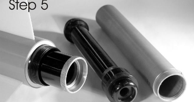
When ready to fly, insert a motor into the motor tube. The HAMR system works with most motor brands and types. In this case, an Aerotech (TM) motor is being inserted into the motor tube.
