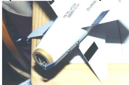
**Figure 2 - Bullpuppy Aluminum Retainer Clip**
